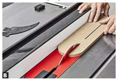
To prevent the slot from closing up around the blade and riving knife, glue a kerf-wide spacer into the end of the slot, making sure there's still adequate clearance for the riving knife [**Photo C**, **below**]. You now have a zero-clearance insert with a perfectly matched opening for your riving knife.
